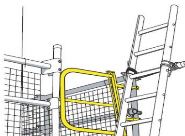
Access ladders must be tied and extend at least 1 m above the landing point to provide a secure handhold.
